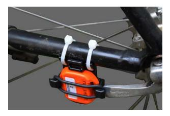
Check tie tension and clip alignment then cut excess tie.
