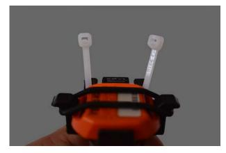
Slide a cable tie through each small slot in tag clip
