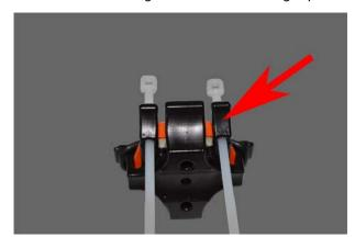
Place indicated curves of clip on lower section of chainstay at required distance and pull ties firm.
